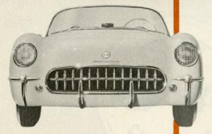
WINDSHIELD - Chrome-bound, onepiece, curved Safety Plate Glass; 55degree slant. HOOD-Glass-fiber hood. with hinges at front. HEADLIGHTS-Recessed in fenders; parking lights beside ends of radiator grille. RADIATOR GRILLE-Chrome airscoop radiator grille. FRONT GUARDS—Chrome grille guard; chrome fender guards. FRONT SUSPENSION-Knee Action, with direct double-acting shock absorbers, and ride stabilizer, STEERING-Full anti-friction steering gear, Center-Point Steering linkage.
