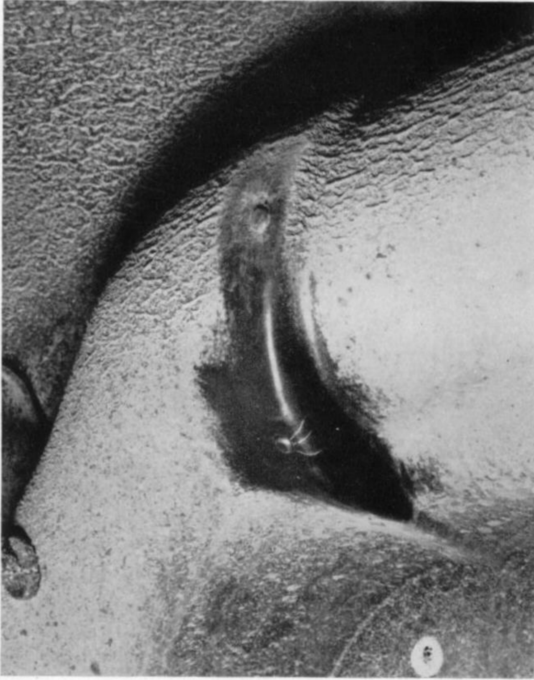
Fig. 45. Wing support, left front cracked on delivery.
