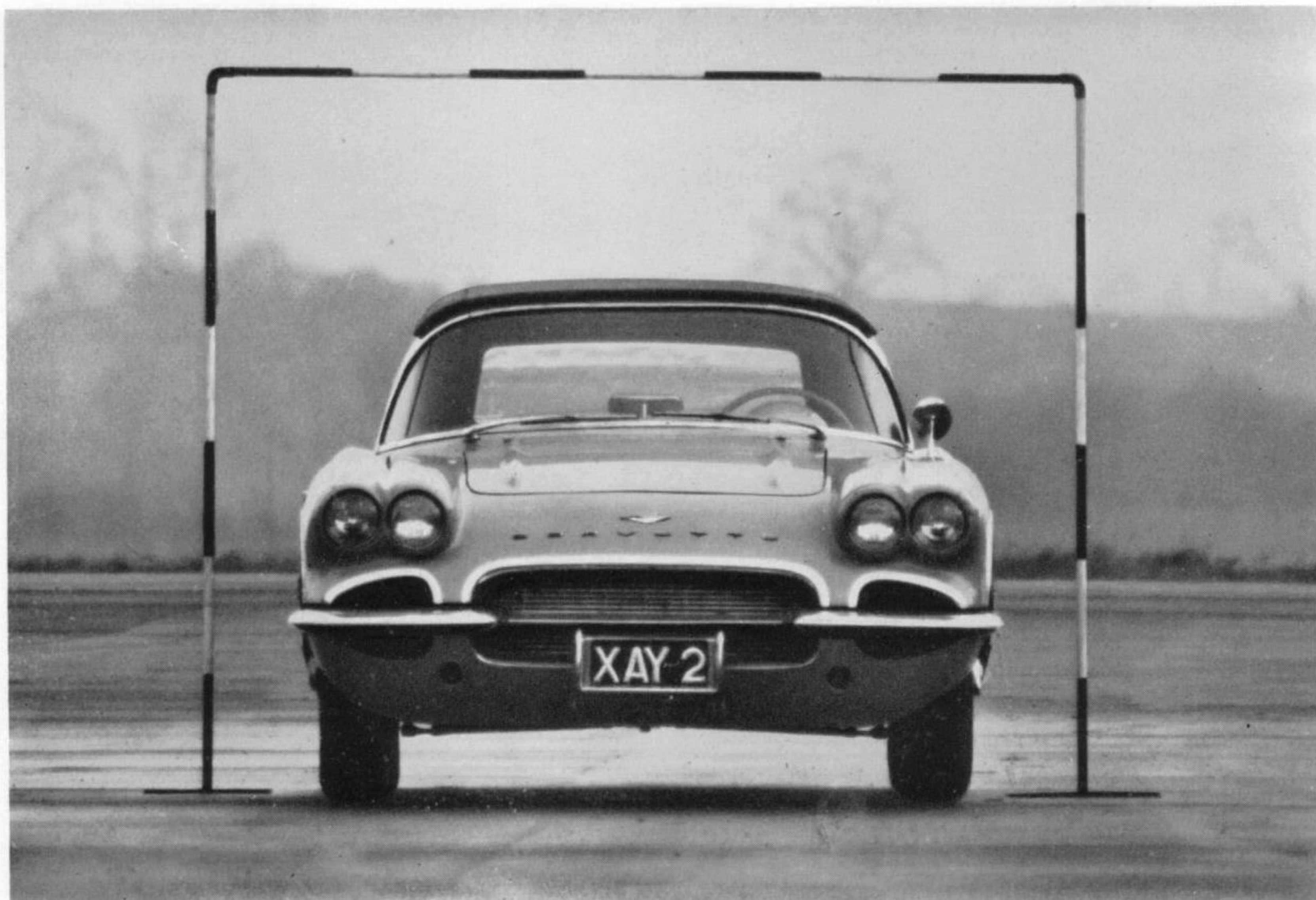
Fig. 2. Front view. Scale bars marked at 1 ft. intervals, camera 200 ft. from windscreen.
