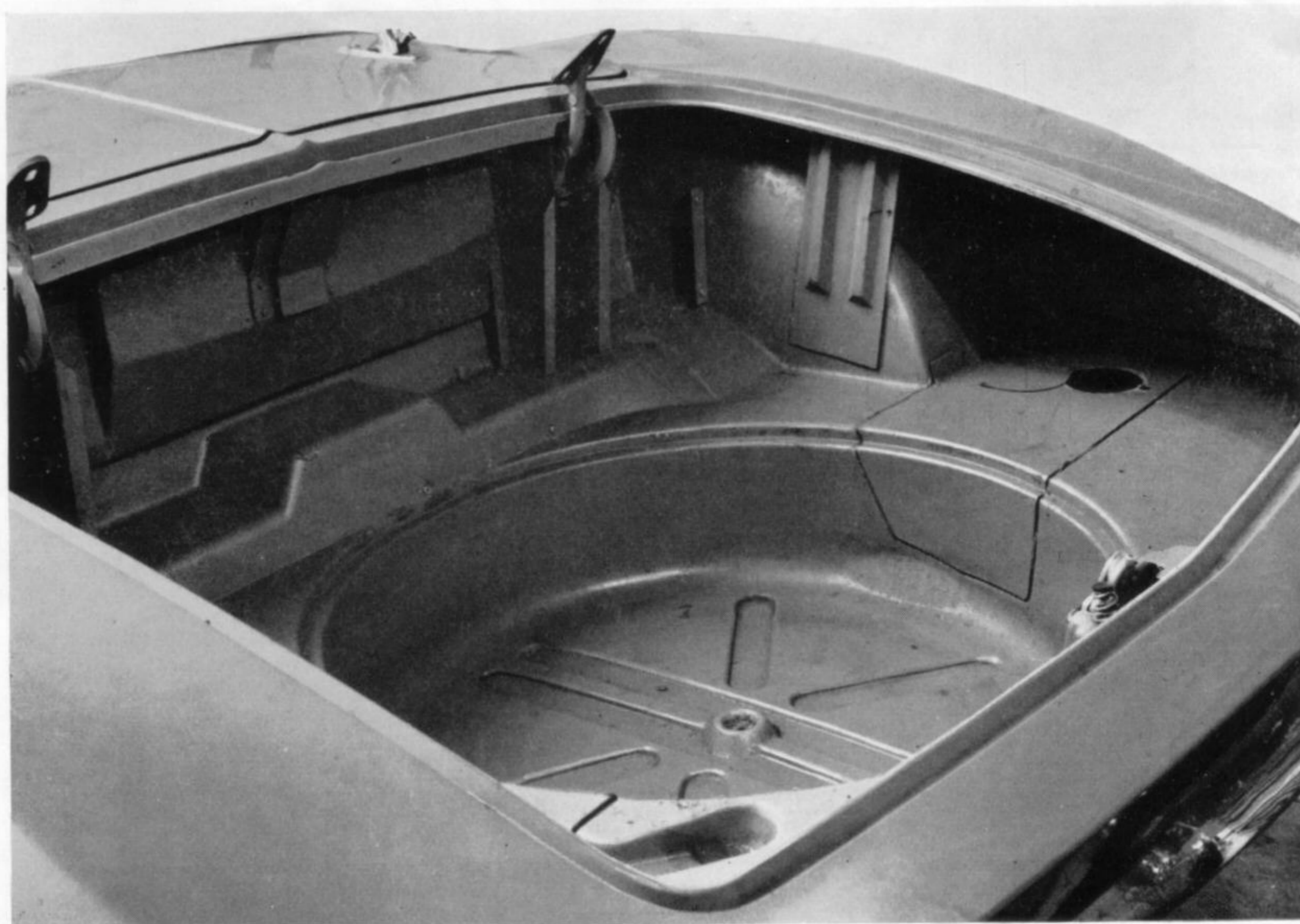
Fig. 71. Luggage compartment with trim removed.
