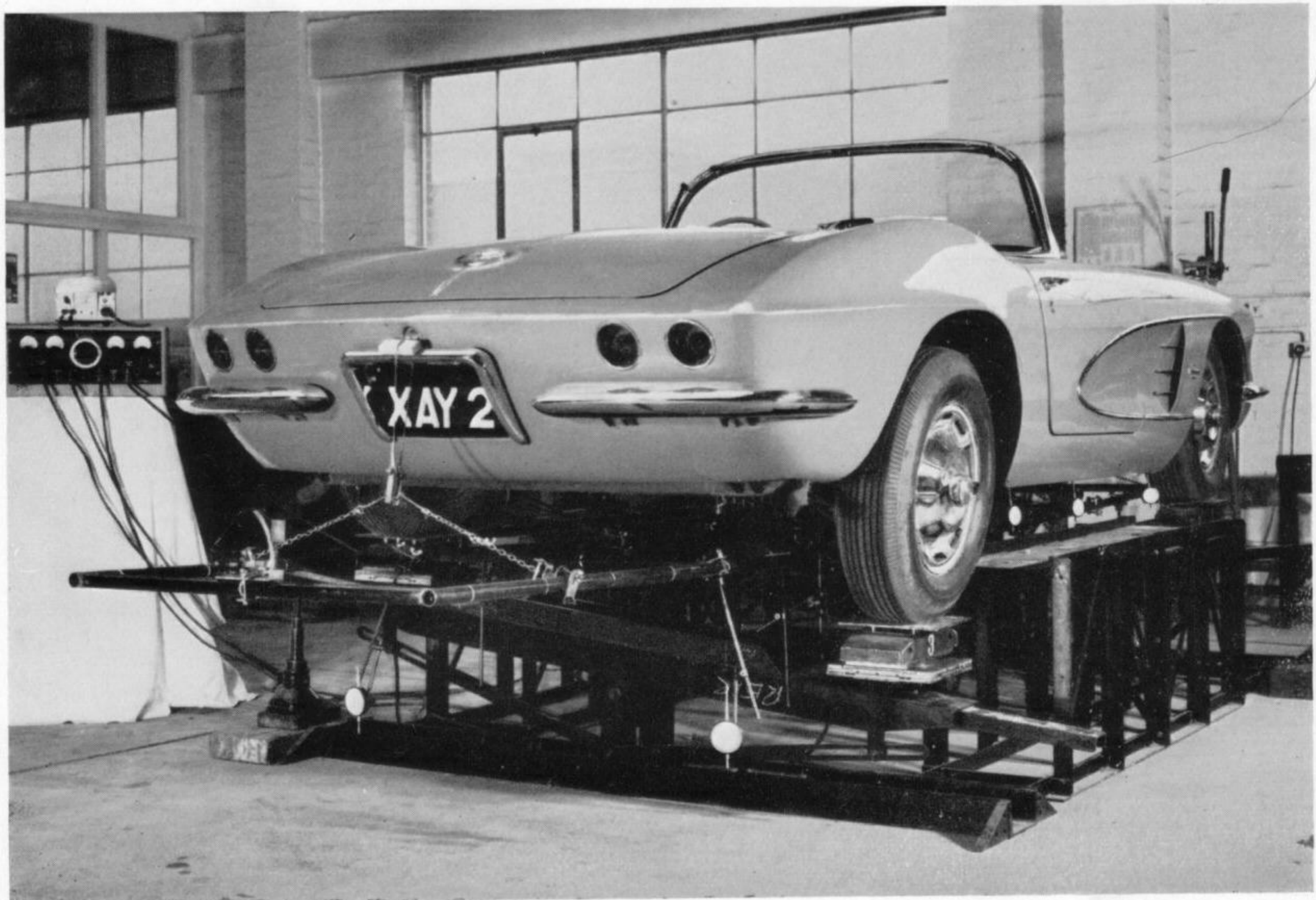
Fig. 38. Vehicle mounted for torsional testing.
