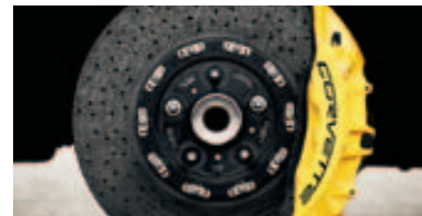
Yellow calipers 1 shown with Brembo carbon ceramic brakes for Z06 with Z07 Package and ZR1.
